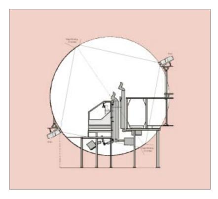
The front of the lens coincides the surface of the dome. Each projector can display an image on one half of a dome.
