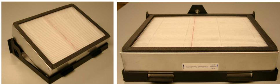
Insert the frame with the fresh filter pad into the illumination unit.
