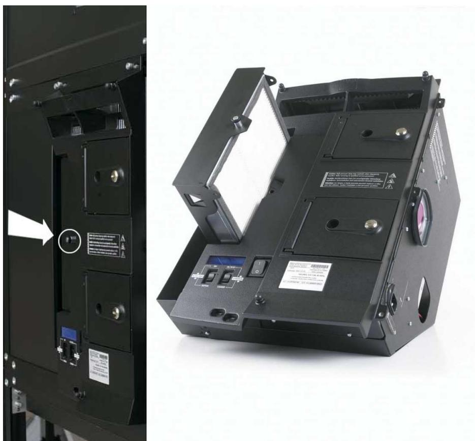
The connection between the frame of the filter pad module and the cover of the fan inside the illumination unit is not only provided by the bolt but also by a hinge: two "noses" of the frame are positioned into the respective recesses of the fan cover in the illumination unit.
